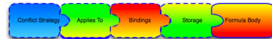
**Fig. 1. Formula components - dashed lines mean optional component**
